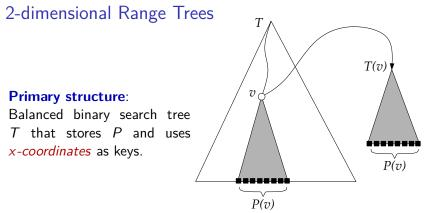
Each node v of T stores an **associate structure** T(v):
