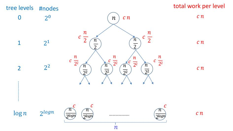
• cn operations on each tree level,  $\log n$  levels, total work is  $cn \log n \in \Theta(n \log n)$
