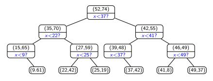
Key idea: The x-coordinate stored for splitting can be *different* from the x-coordinate of the stored point.
