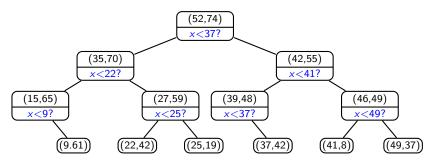
Key idea: The *x*-coordinate stored for splitting can be *different* from the *x*-coordinate of the stored point.
