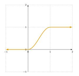
A sin-squared window, used in signal processing, can be described by
