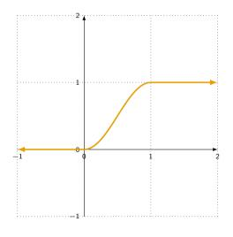
A sin-squared window, used in signal processing, can be described by the following piecewise function:
