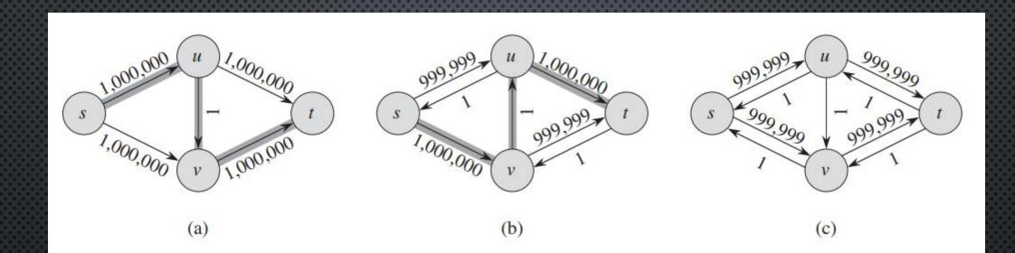
**Figure 26.7** (a) A flow network for which FORD-FULKERSON can take  $\Theta(E \mid f^* \mid)$  time, where  $f^*$  is a maximum flow, shown here with  $|f^*| = 2,000,000$ . The shaded path is an augmenting path with residual capacity 1. (b) The resulting residual network, with another augmenting path whose residual capacity is 1. (c) The resulting residual network.
