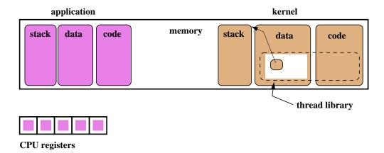
Each OS/161 thread has two stacks, one that is used while the thread is executing unprivileged application code, and another that is used while the thread is executing privileged kernel code.
