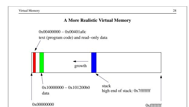
This diagram illustrates the layout of the virtual address space for the OS/161 test application user/testbin/sort
