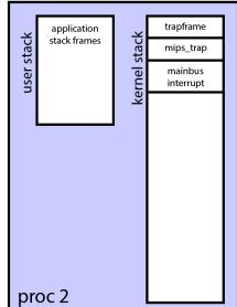
The interrupt handler returns to mainbus\_interrupt.
