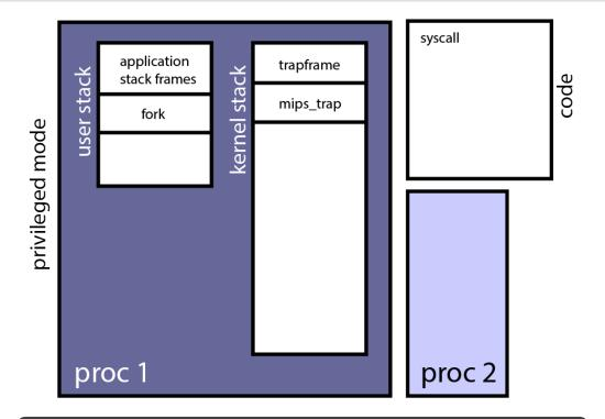
mips\_trap determines exception is a system call. Calls syscall, a kernel function to dispatch the correct function.
