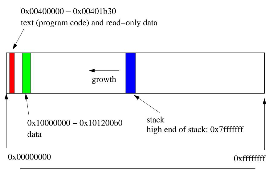
This diagram illustrates the layout of the virtual address space for the OS/161 test application testbin/sort
