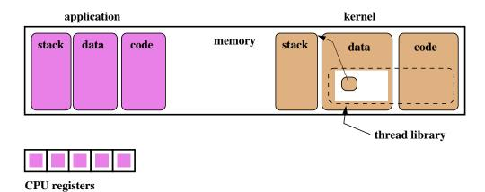
Each OS/161 thread has two stacks, one that is used while the thread is executing unprivileged application code, and another that is used while the thread is executing privileged kernel code.
