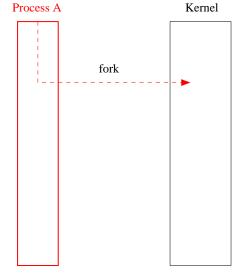
Parent process (Process A) requests creation of a new process.
