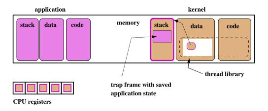
While the kernel handles the system call, the application's CPU state is saved in a trap frame on the thread's kernel stack, and the CPU registers are available to hold kernel execution state.
