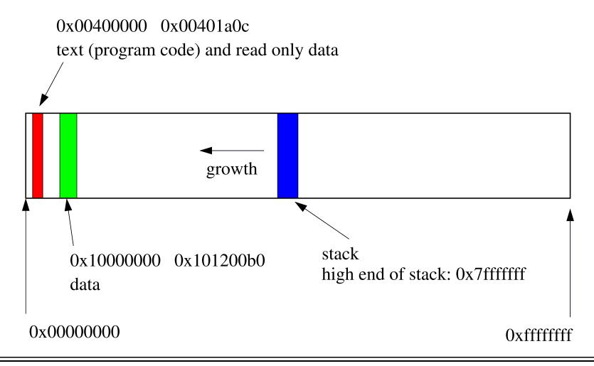
This diagram illustrates the layout of the virtual address space for the OS/161 test application user/testbin/sort
