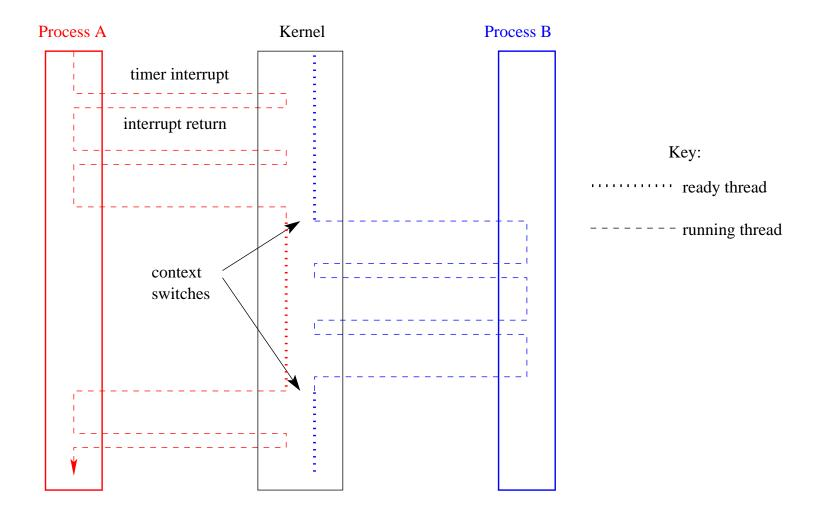
Two process' threads timesharing a single CPU.
