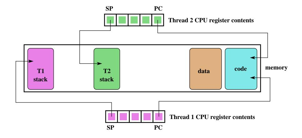
Conceptually, each thread executes sequentially using its private register contents and stack.
