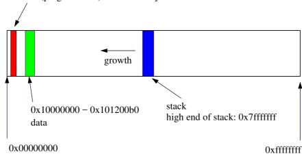
This diagram illustrates the layout of the virtual address space for the OS/161 test application user/testbin/sort
