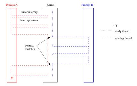
Two process' threads timesharing a single CPU.
