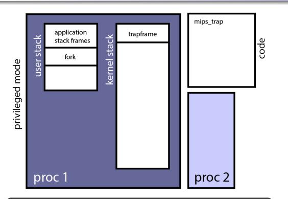
After saving the state common\_exception calls mips\_trap to determine what kind of exception was raised. For a system call, turn interrupts back on.
