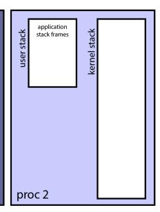
Thread context is restored from trapframe. Switch from kernel to user stacks. Switch to unprivileged mode. User code continues execution.
