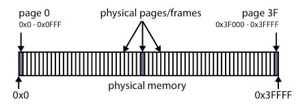
Physical memory is divided into fixed-size chunks called **physical pages**, or, **frames**. Physical addresses, in this example, are 18bits. Physical page size, in this example, is 4KB. There are  $2^{18}/2^{12}=2^6=64$  frames of physical memory.
