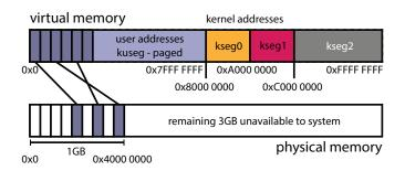
User virtual memory, kuseg, is paged. The kernel maintains the page-to-frame mappings for each process. The TLB is used to translate kuseg virtual addresses to physical ones.
