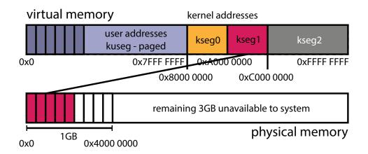
Addresses within kseg1 are for accessing devices. To translate kseg1 addresses to physical ones **subtract** 0xA000 0000 from the virtual address.
