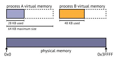
In this example, virtual addresses are 16 bits maximum virtual memory size is 64KB. Physical memory is 18 bits addressable, therefore physical memory is 256KB (in hexadecimal 0 to 0x3FFFF).
