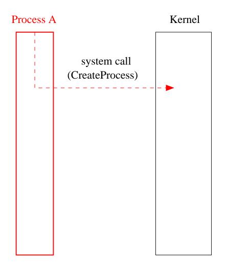
Parent process (Process A) requests creation of a new process.
