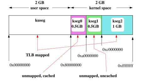
In OS/161, user programs live in kuseg, kernel code and data structures live in kseg0, devices are accessed through kseg1, and kseg2 is not used.
