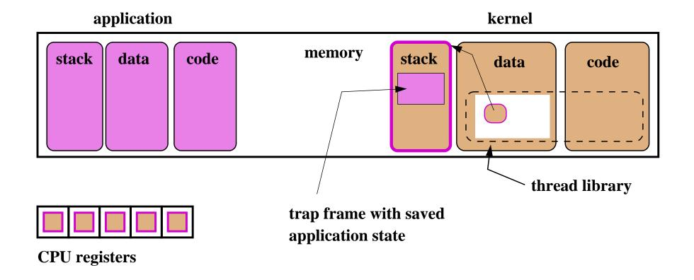
While the kernel handles the system call, the application's CPU state is saved in a trap frame on the thread's kernel stack, and the CPU registers are available to hold kernel execution state.
