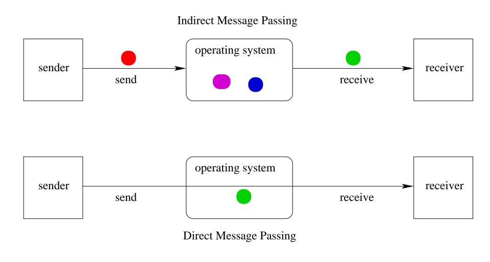
If message passing is indirect, the message passing system must have some capacity to buffer (store) messages.
