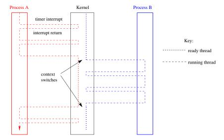
Two process' threads timesharing a single CPU.
