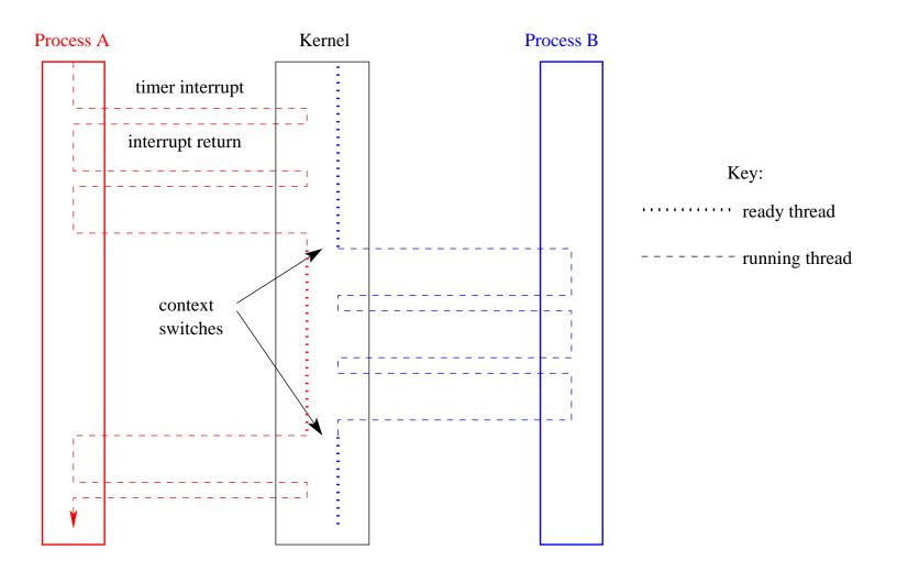
Two process' threads timesharing a single CPU.
