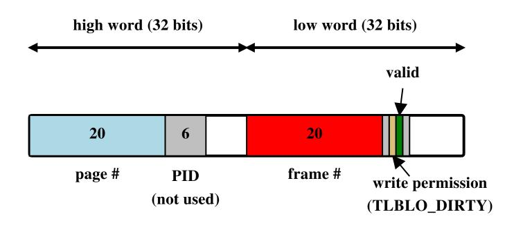
The MIPS TLB has room for 64 entries. Each entry is 64 bits (8 bytes) long, as shown. See kern/arch/mips/include/tlb.h
