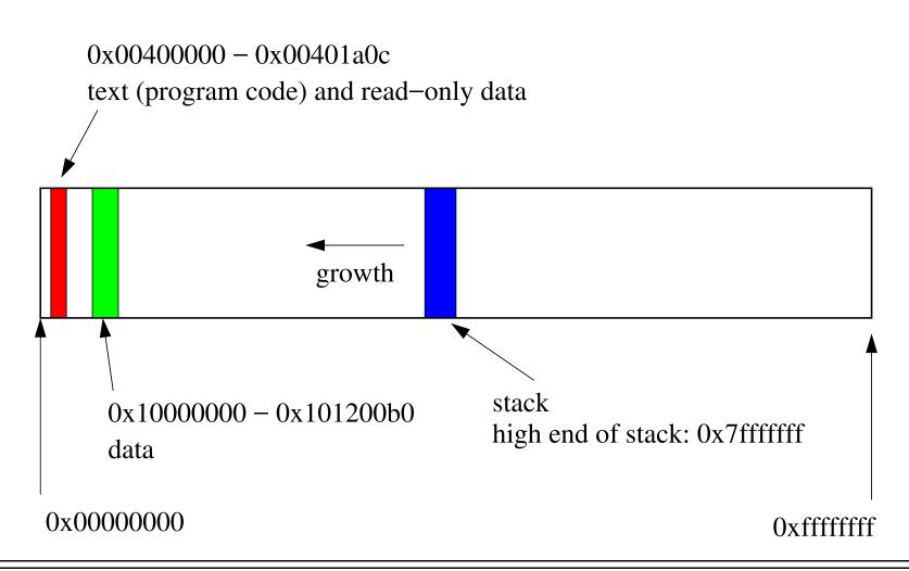
This diagram illustrates the layout of the virtual address space for the OS/161 test application user/testbin/sort
