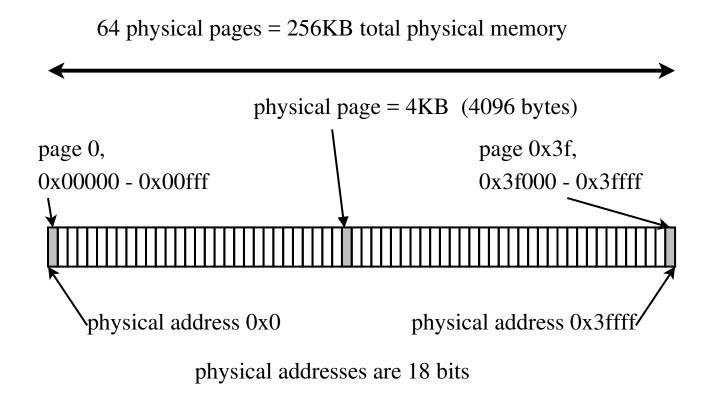
Physical memory is divided into fixed-size chunks called *frames* or *physical pages*. In this example, the frame size is  $2^{12}$  bytes (4KB).
