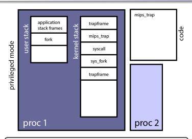
mips\_trap determines which exception has been raised. In this case, a timer interrupt.
