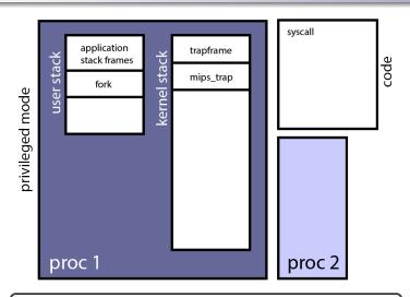
mips\_trap determines exception is a system call. Calls syscall, a kernel function to dispatch the correct function.
