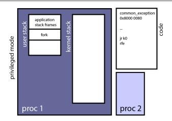
mips\_trap returns to common\_exception. The trapframe data is restored. Switch from kernel to user stack. Switch to unprivileged mode (rfe). User code continues execution.
