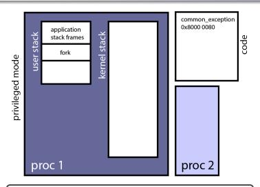
Exception is raised, the CPU executes common\_exception. The CPU goes into privileged mode and interrupts are turned off. Switch from user to kernel stack. Save trapframe.
