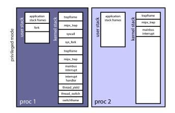
The interrupt handler returns to mainbus\_interrupt.
