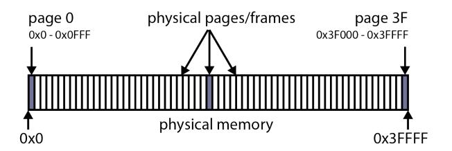
Physical memory is divided into fixed-size chunks called **physical** pages, or, **frames**. Physical addresses, in this example, are 18bits. Physical page size, in this example, is 4KB.
