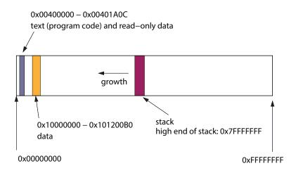
This is the layout of the virtual address space for the OS/161 test application user/testbin/sort. Note that it requires a total of 1.2MB divided between code, data, and stack segments. However, the virtual memory is 4GB in size (32bit addressing).
