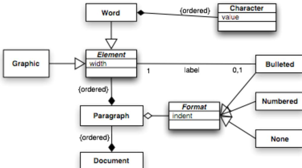
In this model, for scenario (a) the selection of paragraphs would be assigned a new Bulleted Format,
