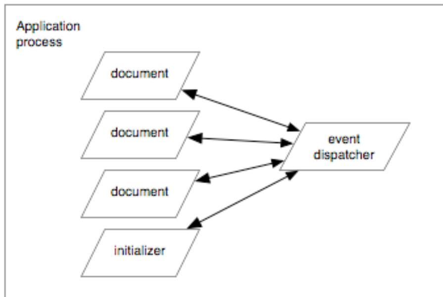
For scenario (a) the event dispatcher would send the user's request to the appropriate document thread. (Changes would be sent to the presentation layer, not shown.) Of course the operations in scenario (a) would take place so quickly that multithreading would have no effect whatever on performance.
